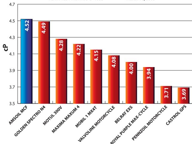
The high temperatures and tight tolerances common to motorcycle applications also affect viscosity. The High Temperature/High Shear (HTHS) Test (ASTM D-4683) measures a lubricant's viscosity under severe high temperature and shear conditions. The more resistant an oil is to high-temperature viscosity loss, the better it protects, and even a HTHS difference of 0.1 cP makes a significant difference.
