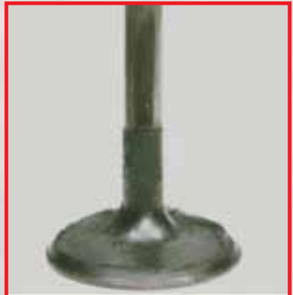
Intake valve after P.i. treatment
