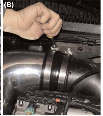
Once you have aligned the cast intake to the step hose, continue to press the intake into the hose (A) The power-band on the intake side is semi-tightened to hold the intake in place (B).
