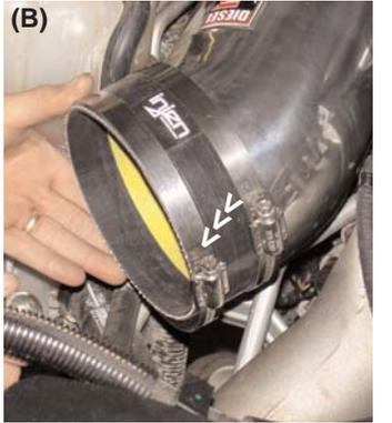
Place one power-bands over the 5 1/2" straight hose and tighten the clamp to prevent the hose from slipping off (A). Place the remaining power-band over the opposite end of the 5 1/2" straight hose but do not tighten this clamp at this point (B).
